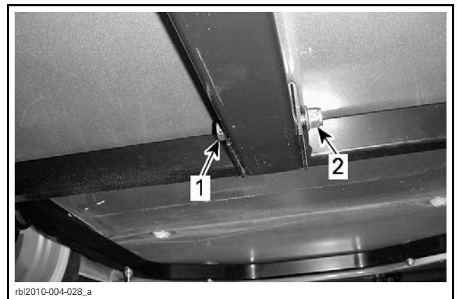
1. M10 x 75 hexagonal flanged bolt [P4] 2. M10 elastic flanged nut [P3]
