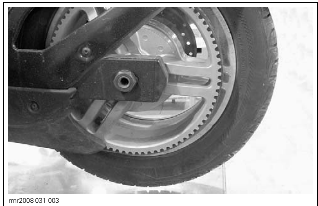
TYPICAL - SWING ARM ALIGNS WITH A SPOKE
