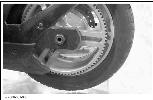
TYPICAL - SWING ARM ALIGNS WITH A SPOKE
