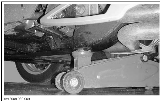
TYPICAL - LIFT BY THE FRAME
