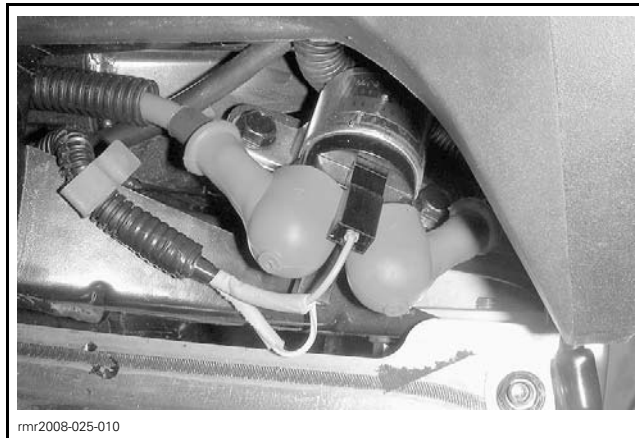
STARTER SOLENOID (RH FUEL TANK COVER REMOVED)
