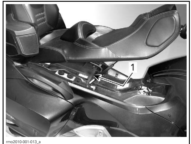
1. Rear fuse box (master)
