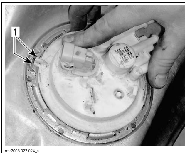
TYPICAL - PUMP INDEXING 1. Index tab with notch
