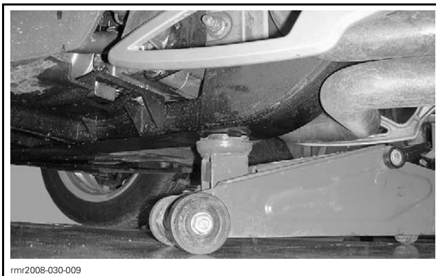
TYPICAL - LIFT BY THE FRAME
