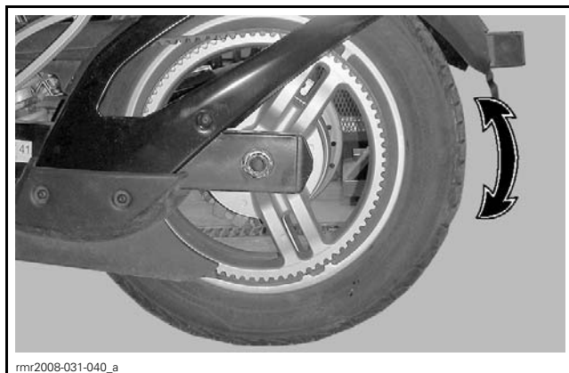
TYPICAL - SWING ARM ALIGNS AT MIDWAY OF SPOKES
