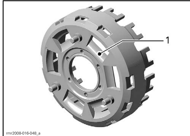
1. Inspect spring cavity
