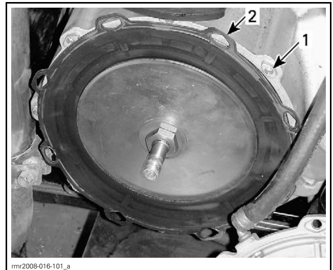
1. Mounting lugs 2. Diaphragm rotated out of lugs
