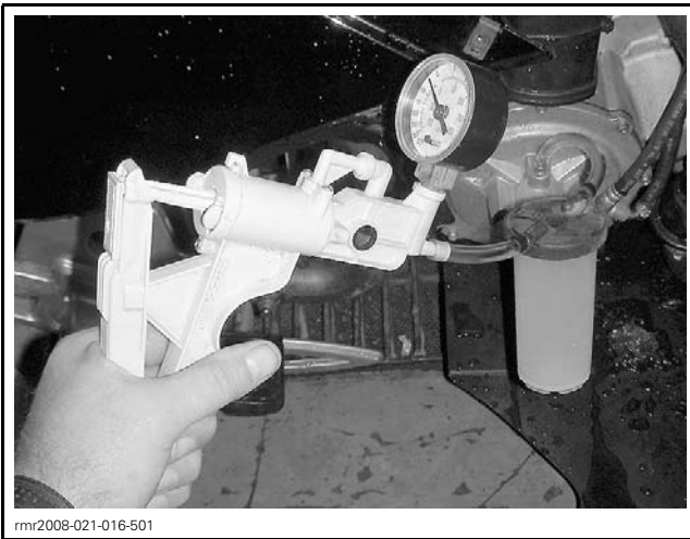
ACTIVATE PUMP UNTIL FLUID REACHES CLUTCH RESERVOIR
