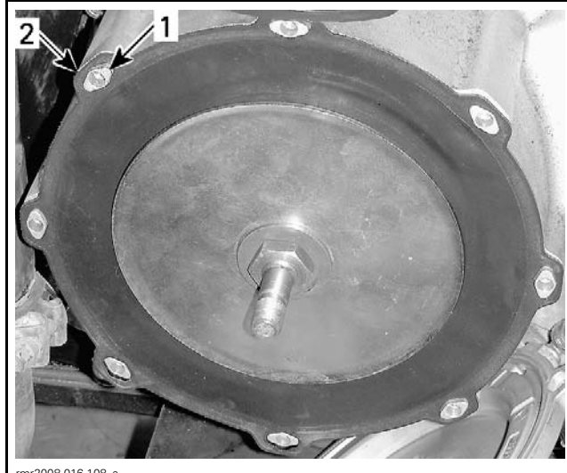
1. Mounting lug 2. Diaphragm slot inserted on lugs
