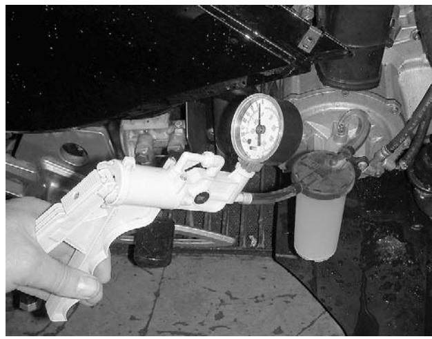
TYPICAL - PUMP AND REMOTE RESERVOIR INSTALLATION
