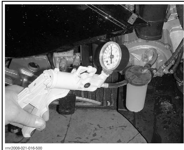
TYPICAL - PUMP AND REMOTE RESERVOIR INSTALLATION
