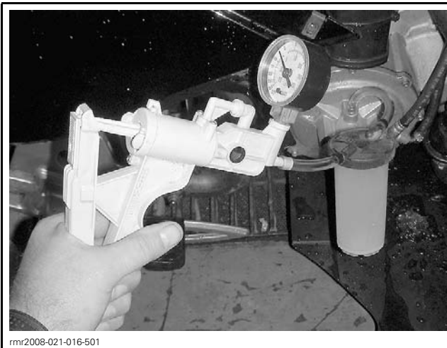
ACTIVATE PUMP UNTIL FLUID REACHES CLUTCH RESERVOIR
