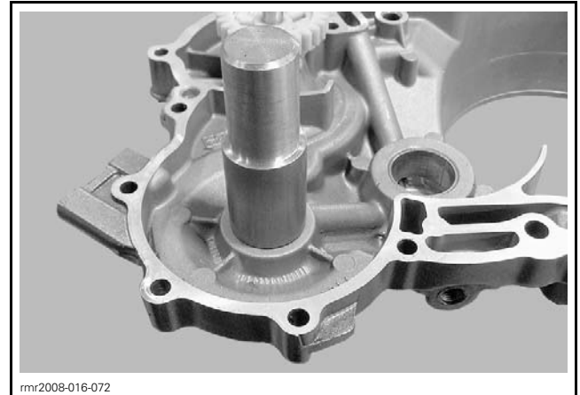
PLAIN BEARING INSTALLER — BALANCE SHAFT SUPPORT BEARING
