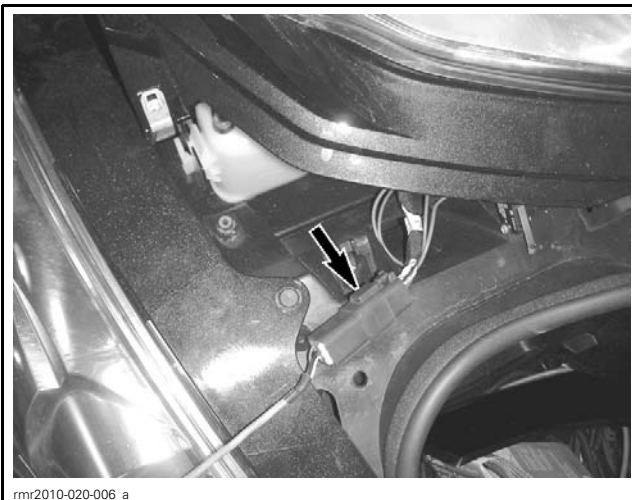
TYPICAL - MPI-2 CONNECTION TO VEHICLE COMMUNICATION CONNECTOR
