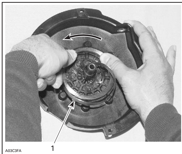
TYPICAL 1. Outer end into guide notch
