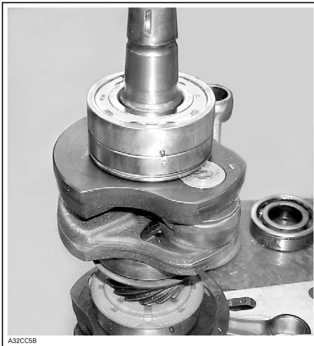
PTO SIDE BEARING FILLED WITH ISOFLEX GREASE
