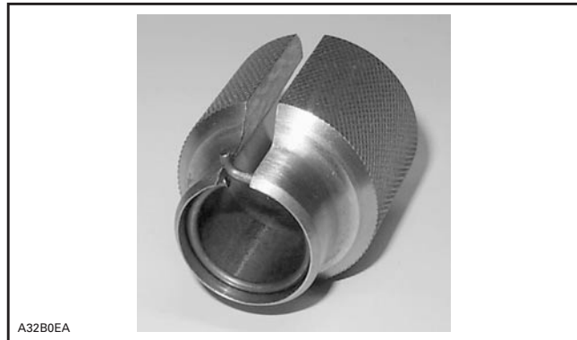
CIRCLIP READY TO BE INSTALLED ON PISTON
