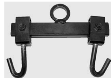
N -> 2-stroke engine lifting tool (P/N 529 035 940)
