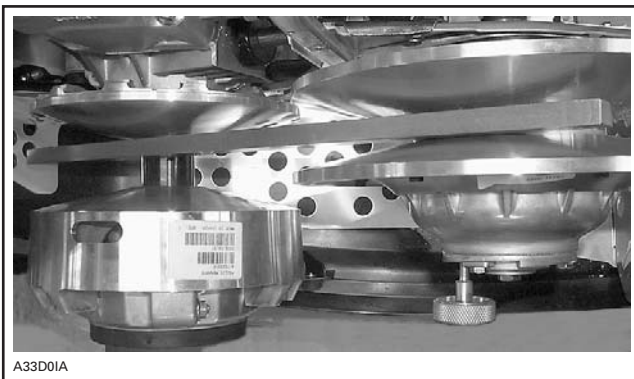
ALIGNMENT BAR IN PULLEYS
