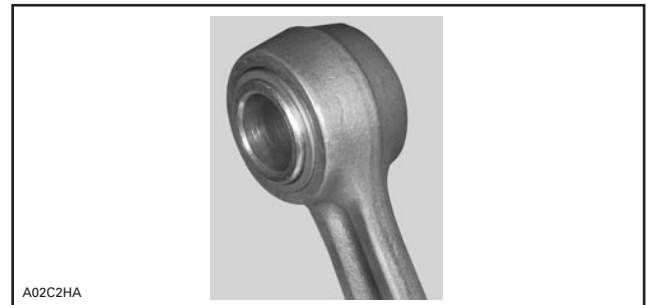
TYPICAL — CAGELESS BEARING AND SLEEVE INSTALLED
