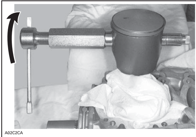
TYPICAL — PISTON PIN EXTRACTION
