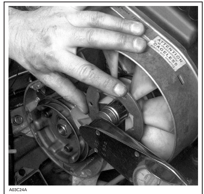
TYPICAL — TORQUE FAN NUT USING HOLDER WRENCH
