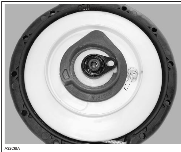
FREE PORTION INSERTED INTO SHEAVE
