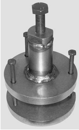
Countershaft bearing remover (P/N 529 035 812)
