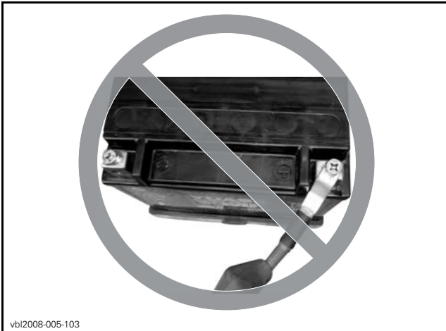
WRONG WAY OF SECURING THE POSITIVE (+) POST
