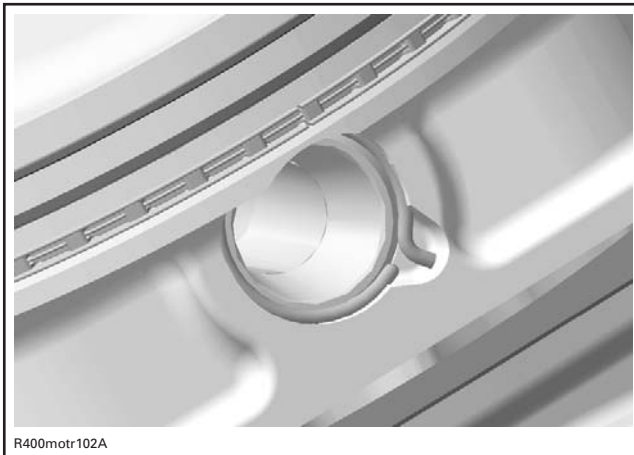
CORRECT POSITION OF THE PISTON CIRCLIP
