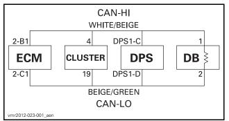
CLUSTER: Multifunction Gauge DB: Diagnostic Connector ECM: Engine Control Module DPS: Dynamic Power Steering WHITE/BEIGE: (wire color code) BEIGE/GREEN: (wire color code)
