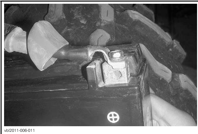
TYPICAL - CORRECT WAY OF SECURING POSITIVE (+) POST
