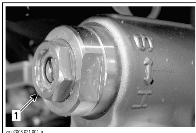
COMPRESSION - HIGH SPEED 1. Compression adjuster (17 mm wrench)
