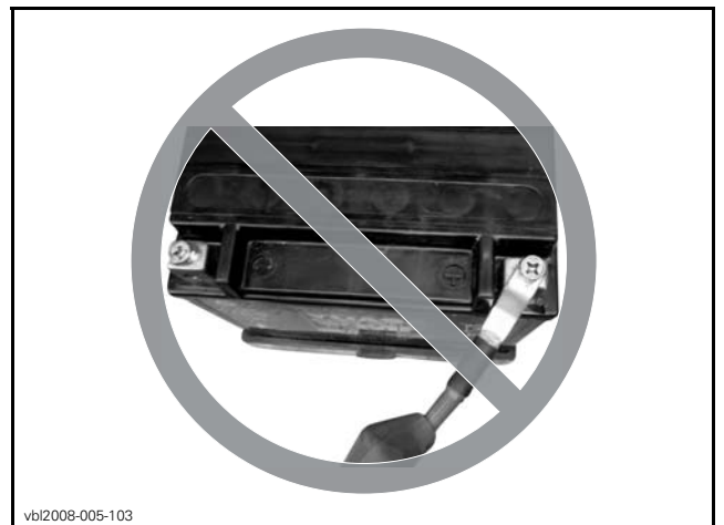
WRONG WAY OF SECURING THE POSITIVE (+) POST
