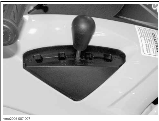
vmo2006-007-007 TYPICAL - TRANSMISSION LEVER
