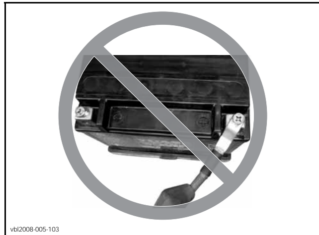
WRONG WAY OF SECURING THE POSITIVE (+) POST
