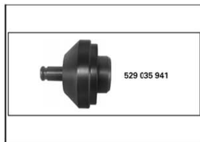
Output shaft seal installer P/N 529 035 941 Mandatory 400 engines Use with handle 420 877 650
