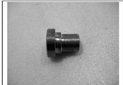
Needle bearing installer P/N 529 036 109 Recommended DS 450
