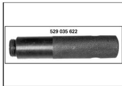
Cover remover P/N 529 035 622 Recommended DS 650
