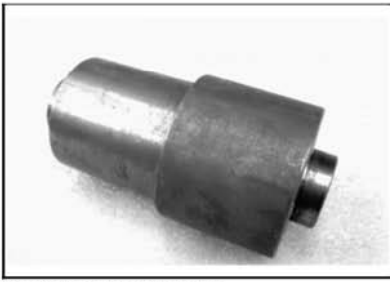
Bearing remover/installer P/N 529 035 918 Mandatory Outlander, Renegade, DS 450
