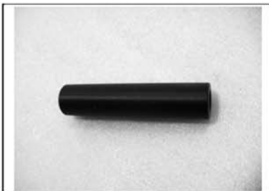
Oil seal installer P/N 529 036 070 Recommended 449 engine Insertion jig for gearshift shaft.
