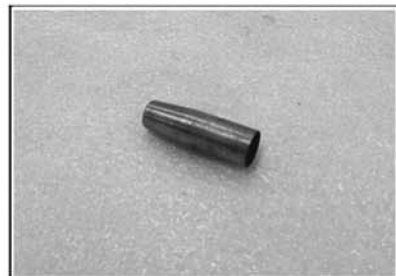
Protection sleeve P/N 529 036 071 Recommended 449 engine Gearshift shaft
