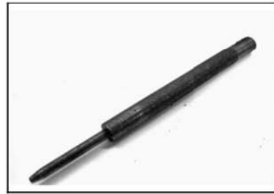
Valve guide remover 5 mm P/N 529 035 924 Recommended 400, 500, 650, 800 engines
