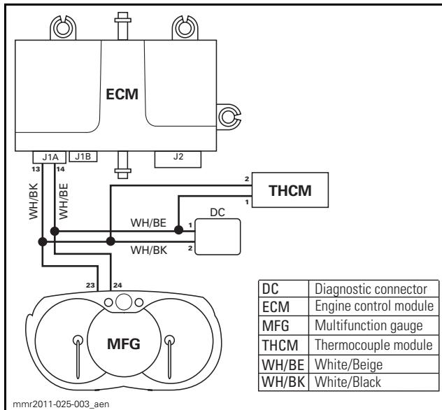
Fault codes are broadcasted to the CAN bus. They can be displayed:
