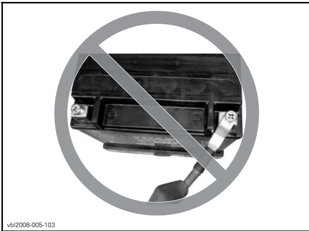
WRONG WAY OF SECURING THE POSITIVE (+) POST
