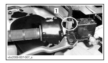
Install mirror adaptor [1] between handlebar support and RH mirror.
