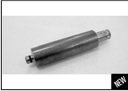
Bearing installer P/N 529 036 078 Recommended 449 engine Use with handle 420 877 650
