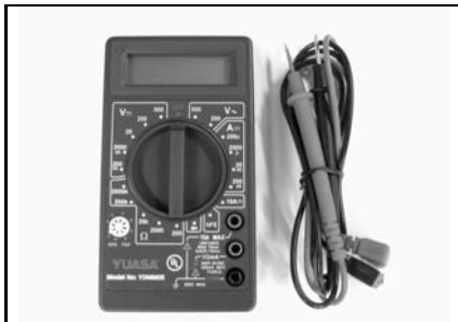
Digital multimeter (basic model) P/N 529 035 774 Recommended
