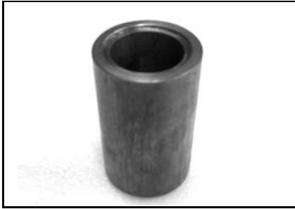
PTO cover oil seal installer P/N 529 036 033 Recommended V-490, V-660 & V-810 engines
