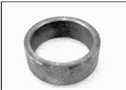
Crankcase support (MAG side) P/N 529 035 916 Recommended 330/400 engine
