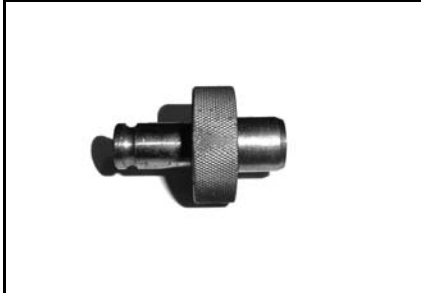
Bearing installer (gearbox) P/N 529 035 762 Recommended V-490, V-660, V-810 engines Use with handle 420 877 650
