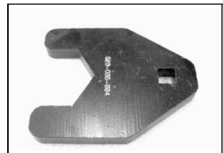
Crow foot P/N 529 035 884 Recommended Rally 200 Rear axle nut
