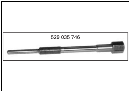
Clutch puller P/N 529 035 746 Mandatory 610/500, V-490, V-660, V-810 engines
