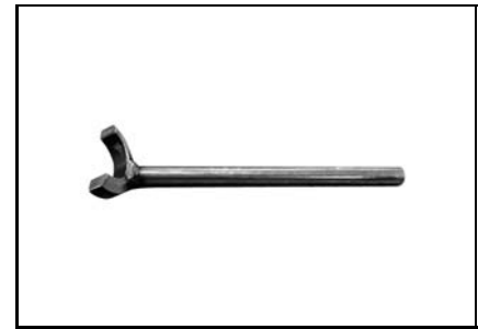
CV joint extractor P/N 529 036 005 Recommended Outlander/Renegade V-660 & V-810
