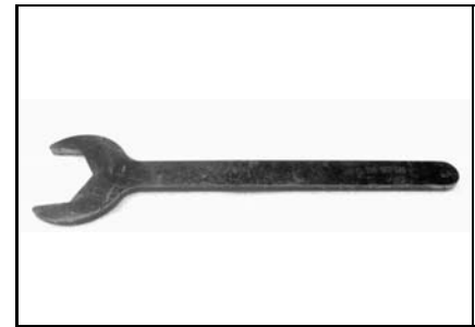
Open wrench 50 mm P/N 529 035 866 Recommended Rally Rally axle nut
