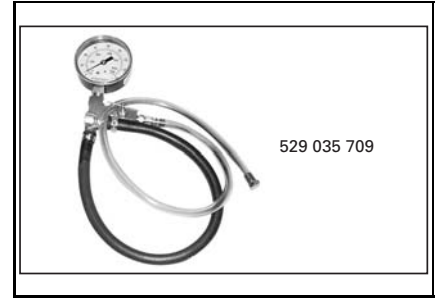
Oil/fuel pressure gauge P/N 529 035 709 Mandatory Injection type engines Use with 529035652, 529035714 & 529036023
