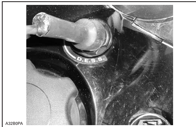
CONNECTED ONTO D.E.S.S. POST
