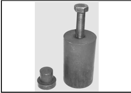
Torque flange remover P/N 529 035 958 Recommended Elite
