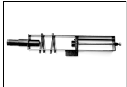
Spring remover P/N 529 036 007 All models To remove coil spring from shock.
