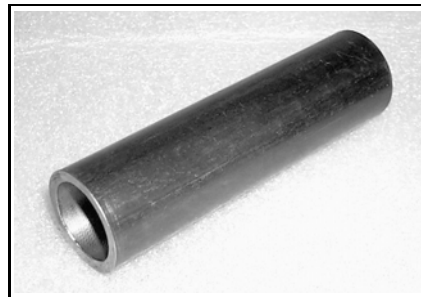
Crankshaft MAG bearing installer P/N 529 035 979 Recommended 493, 593 engines
