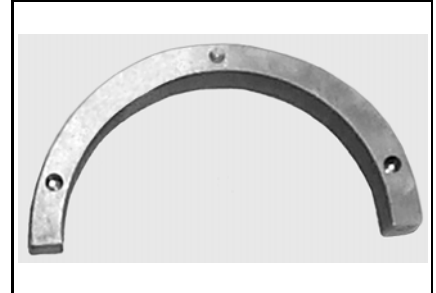
Crankshaft distance gauge P/N 529 035 967 Recommended 593HO, 593 SDI, 693 and 793 To be used with 529035976
