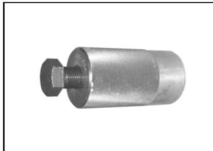
Magneto puller P/N 529 035 748 Recommended All V-twin
