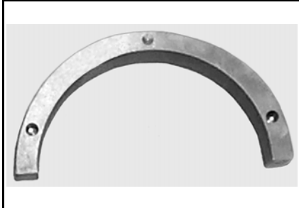
Crankshaft distance gauge P/N 529 035 965 Recommended 552 To be used with 529035876
