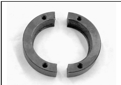
Half-ring puller MAG P/N 420 276 025 Recommended 717 engine To remove crankshaft bearings.
