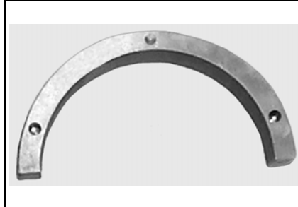
Crankshaft distance gauge P/N 529 035 966 Recommended 493 and 593 To be used with item 529035976
