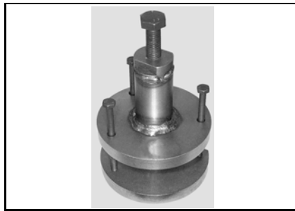
Countershaft bearing remover P/N 529 035 812 Recommended Skandic LT
