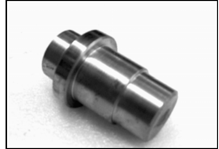
PTO cover plain bearing remover/install. P/N 529 036 032 Recommended V-490, V-660 and V-810 engines
