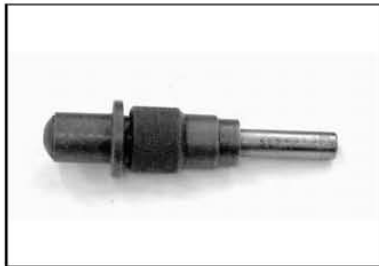
Circlip Insertion Tool 21 mm P/N 529 035 563 Recommended 947 & 947 DI engines Sleeve without groove, P/N 529 035 569 also available.
