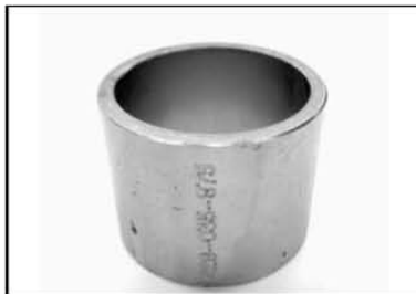
Ball joint installer support P/N 529 035 875 Mandatory REV, RT, Outlander
