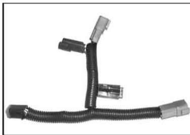
T-harness P/N 529 035 869 Mandatory All DESS equipped
