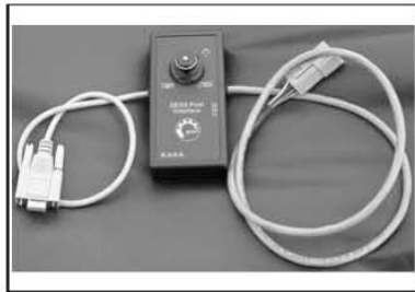
D.E.S.S. Post Interface P/N 529 036 019 Mandatory To program D.E.S.S. keys with the MPI-2.
