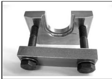
Ball joint extractor P/N 529 035 827 Mandatory REV, RT
