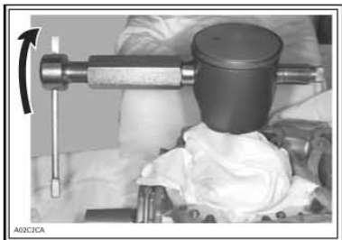
Piston pin puller P/N 529 036 002 Mandatory 995 SDI
